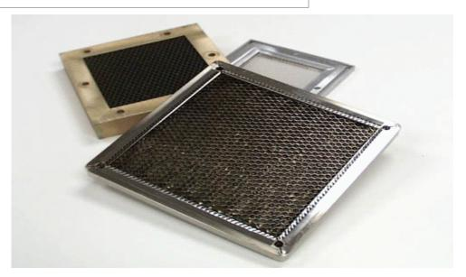
For improved shielding effectiveness and environmental protection, these lightweight aluminum ventilation panels are available tin plated. However, in applications requiring maximum shielding levels and greater weight support, either steel or brass honeycomb shielded vents are recommended. (Refer to page 164, Steel and Brass Honeycomb Shielded Vents, for specifications.)
