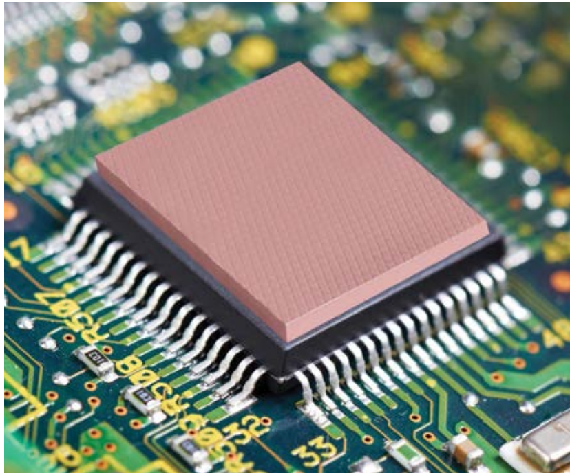
Thermally conductive gap filler pads are cut-to-shape and applied manually to offer thermal properties and high conformability at low clamping forces.
