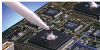
Dispensable gels can be applied manually (Parker Chomerics GEL application, left) or through a semi- or fully automated system for high-volume applications.
